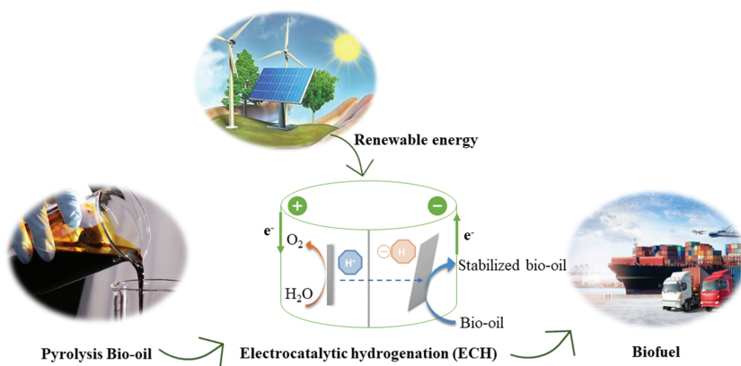
Fig. 7 Schematic of ECH of bio-oil using two electrodes in separate chambers.
