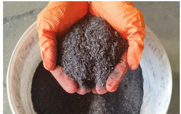
Figure 2: Biochar from contaminated sorghum; “Simone Piazzini monitoring an experiment in the RE-CORD screw pyrolysis unit (SPYRO). Credit: Amr Sanad, RE-CORD R&D engineer
