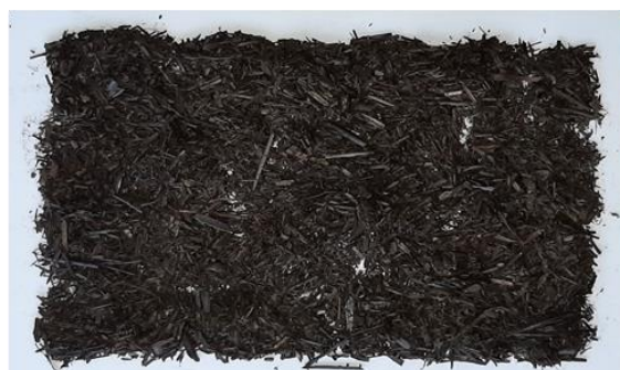
Figure 13: Raw Sorghum feedstock (left) and torrefied sorghum, following continuous pilot scale torrefaction at 280 °C.
