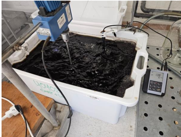
Figure 27: Liquid effluent from Torwash treatment of contaminated Sorghum.
