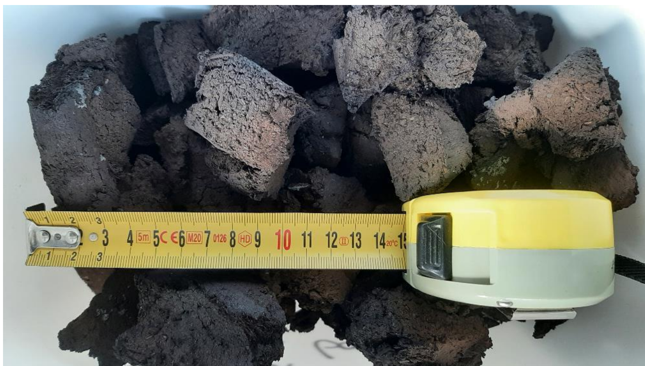
Figure 9: Sorghum solids post-Torwash at 200 °C and pH 2, adjusted with citric acid.
