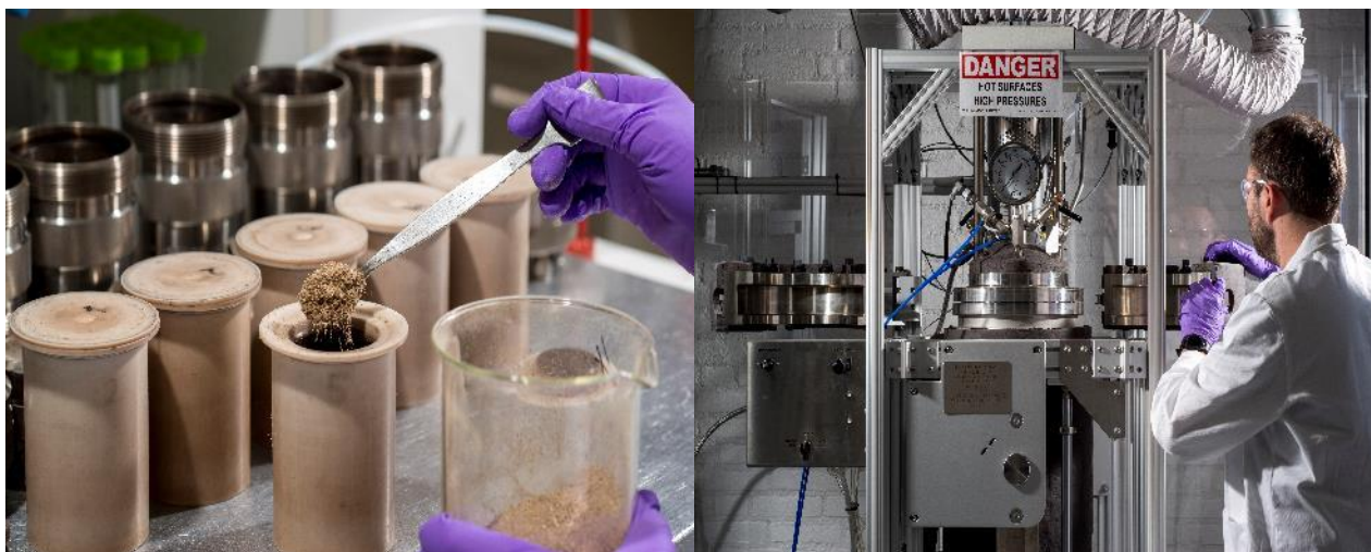
Figure 1: Multiclave apparatus (left) and 30 L autoclave reactor for Torwash pre-treatment optimisation and production experiments, respectively.
