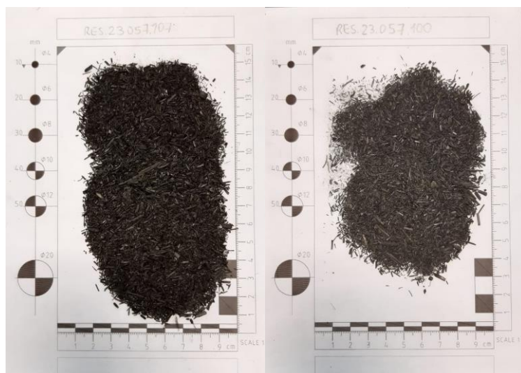
Figure 18: Conventional (left) and oxidative char (right) from sorghum pyrolysis.
