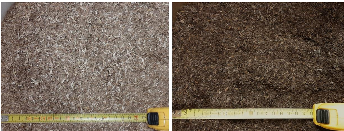
Figure 14: Raw miscanthus feedstock (left) and torrefied miscanthus following continuous pilot scale torrefaction at 285 °C.
