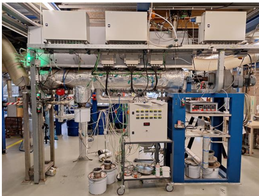
Figure 2: Pilot-scale screw-type reactor used for torrefaction pre-treatment of contaminated biomass (Sorghum and Miscanthus from Lavrion)
