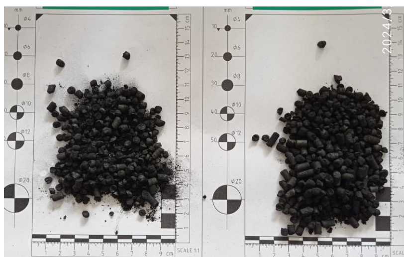
Figure 23: Conventional (left) and oxidative char (right) from Miscanthus (Lavrion) pyrolysis.
